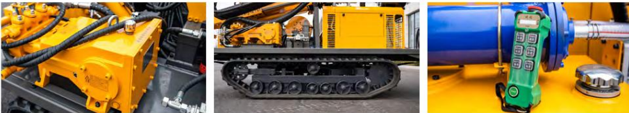
泥浆泵 Mud Pump
