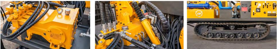
泥浆泵 Mud Pump
